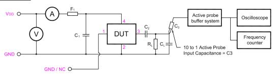
C<sub>1</sub>: 100nF  $C_T = C_L + C_3 (C_3 - Oscilloscope probe capacitance)$  $\textbf{C}_{\text{T}}$  as stated in OSCILLATOR OUTPUT section C₂: ≥1nF  $R_L$ : 10K F  $_{1}$ : A ferrite bead or a resistor between  $22\Omega \sim 47\Omega$  recommended.
